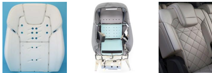
Figure 1: Seat foam (left) and trim cover (middle) which are assembled to a car seat (right).
