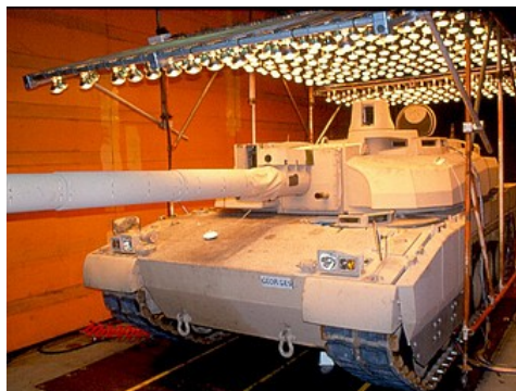
Figure 2: Measurements in thermal wind tunnel S6 in Institut Aérotechnique de Saint-Cyr l'Ecole, Le Cnam
