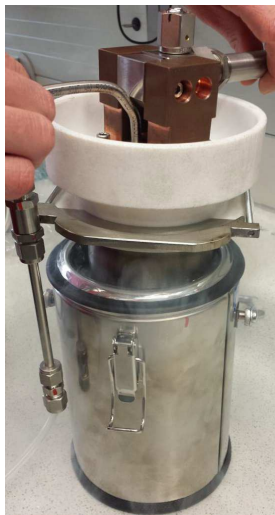
Figure 7 Transport container for LBM with overpressure protection
