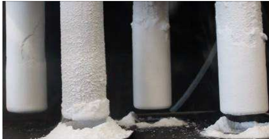
Figure 8. Test of different surface coatings to the CO 2 capture
