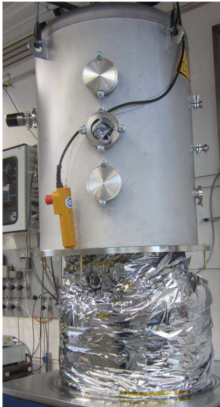
Figure 4 Vacuum bell with radiation shield
