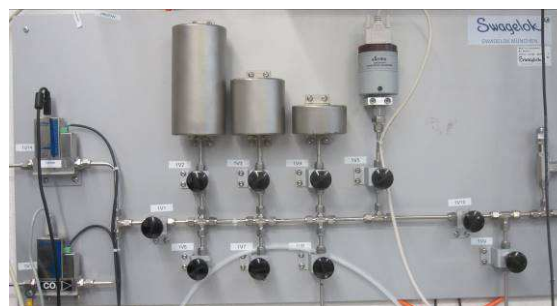
Figure 2 Gas management system
