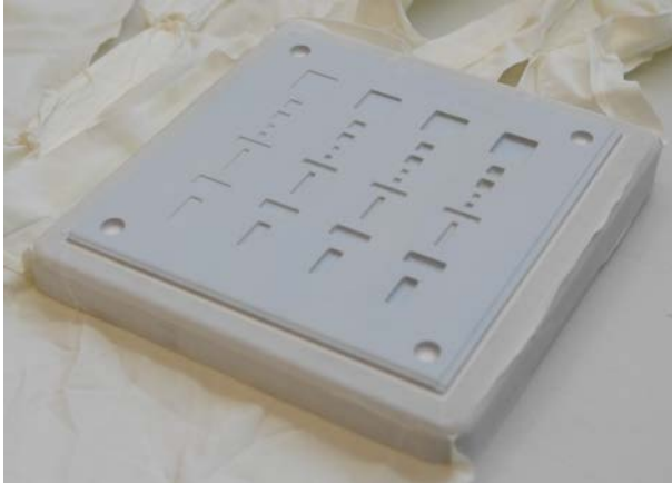
Figure 9: The test substrate sealed into a nitrile glove (after isostatic lamination).
